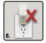
8. If the nightlight did not turn OFF, the GFCI is not working properly.
