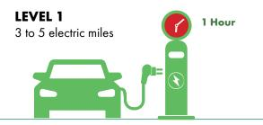
Requires access to a 120-volt outlet in an area where you can recharge the car overnight (or have a qualified electrician install one in a convenient location).
